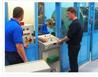
Operations / steel wire armouring of subsea cable
